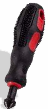
Part No. T CS300 HSS Countersink 12mm 90° on Plastic Handle » Min. cutting size 5mm » Max. cutting size 12mm Suitable for use on steel & wood
