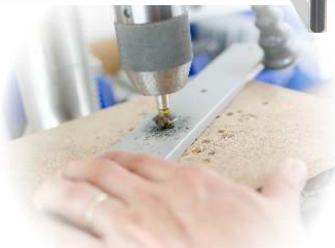
Part No. T CS300 HSS Countersink 12mm 90° on Plastic Handle » Min. cutting size 5mm » Max. cutting size 12mm Suitable for use on steel & wood
